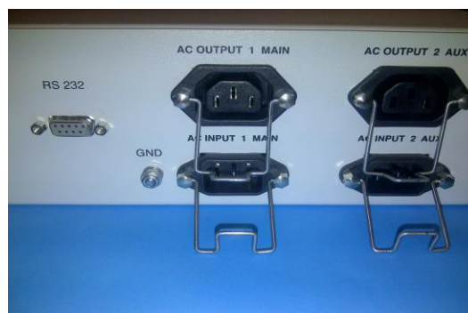
Figure 1-4: Front Panel v5 DB9 modification and rear connectors' distribution overview
