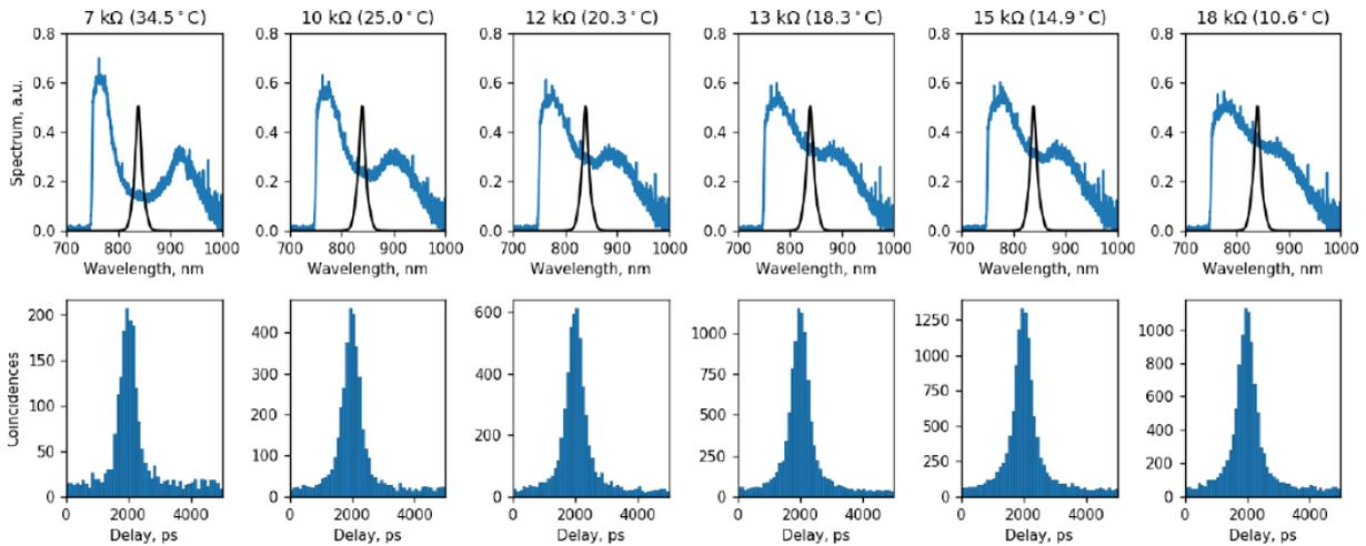
Figure 7. Spectrum (top) and coincidence peak (bottom) for different PPKTP temperatures.
