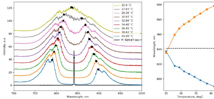
Figure 5. Output spectra obtained for a range of PP-KTP temperatures with a pump wavelength of 420.67nm, illustrating the large bandwidths produced
