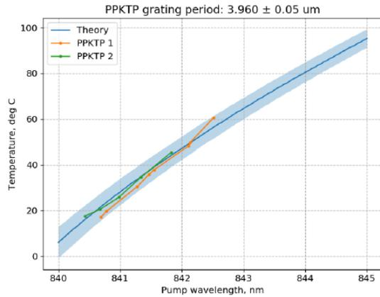
Figure 4. Phase matching temperature Vs wavelength. The ‘Theory’ curve shows calculated values for PPKTP with a grating period of 3.960  $\pm$  0.05 $\mu$ m. For comparison, experimental results for two PPKTP parts are shown in the green and orange curves.
