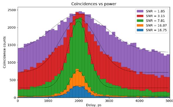
Figure 6. Coincidence peaks for increasing pump powers (blue plot, lower power – purple plot higher power).
