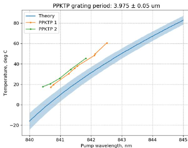
Figure 3. Phase matching temperature Vs wavelength. The ‘Theory’ curve shows calculated values for PPKTP with a grating period of  $3.975 \pm 0.05\mu\text{m}$ . For comparison, experimental results for two PPKTP parts are shown in the green and orange curves.
