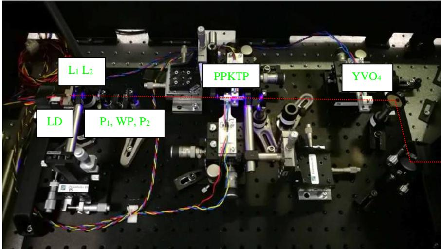
Figure 2. Breadboard entangled photon pair generator. LD is the laser diode pump photon source.  $L_1$  &  $L_2$  are collimation and focus optics.  $P_1$  and  $P_2$  are polarizers and WP is a waveplate for controlling intensity incident on the PPKTP. PPKTP is the two periodically-poled KTP crystals.  $YVO_4$  is the yttrium vanadate crystal.
