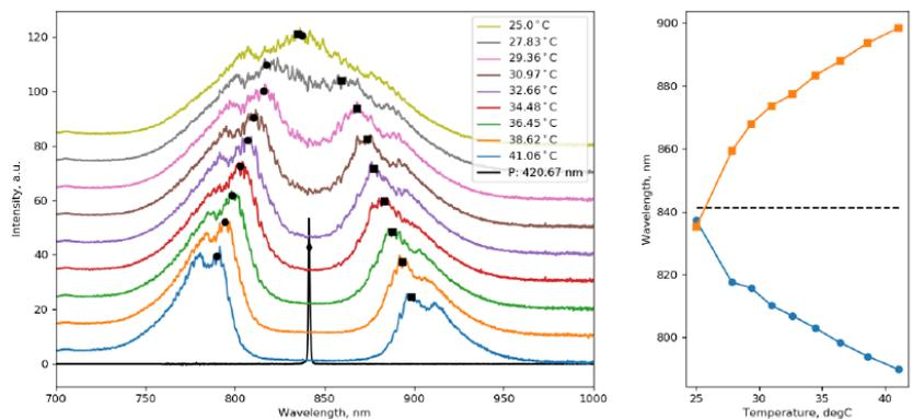
Figure 5. Output spectra obtained for a range of PP-KTP temperatures with a pump wavelength of 420.67nm, illustrating the large bandwidths produced
