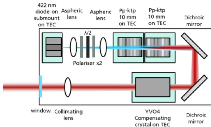
Figure 9. Layout of the packaged entangled photon pairs generator
