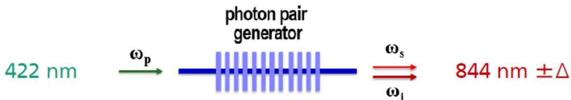
Figure 1. Parametric generation of a signal and idler photon pair at the degenerate wavelength of 844nm from a pump photon at the fundamental wavelength of 422nm.
