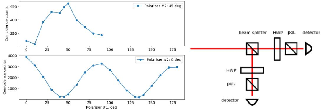
Figure 8. Coincidence counts as a function of the signal polarizer angle for two different settings of idler polarizer (0 degree for the H/V basis case and 45 degree for the diagonal basis).
