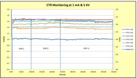
Fig. 5. Time Evolution (min) of the CRT during gamma radiation.
