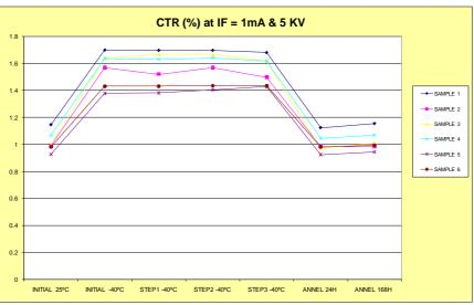
Fig. 4. CTR (at  $I_F$ =1mA and  $V_{RWM}$ = 5KV) after each gamma radiation step.
