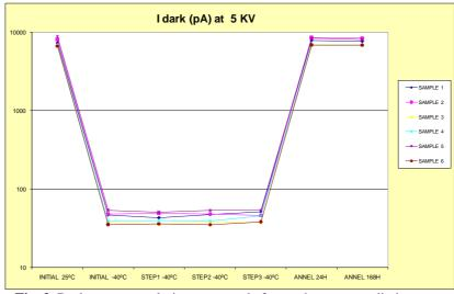
Fig. 3. Dark current evolution measured after each gamma radiation step.
