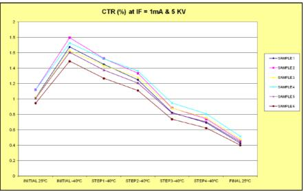
Fig. 8. CTR evolution measured at each intermediate step.
