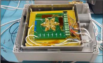
Fig. 1. Radiation testing board with the six HV optocouplers.
