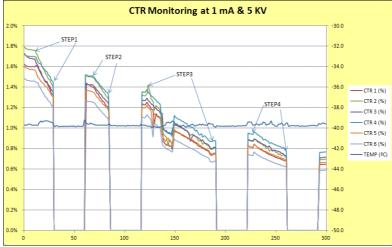
Fig. 6. CTR Time Evolution (min) of the CRT during proton radiation
