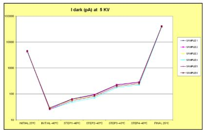
Fig. 7. Dark current plot measured at intermediate steps (Vertical axis scale is logarithmic).
