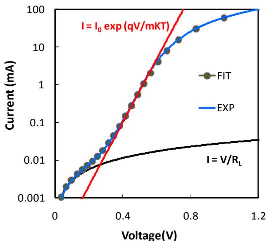
Fig. 3. Experimental (EXP, blue line) and calculated (FIT, grey circles) subthreshold Current-Voltage characteristics for one of the lasers. The black and red lines correspond to the calculated I-V characteristics of the leakage resistance and of the ideal p-n junction, respectively.
