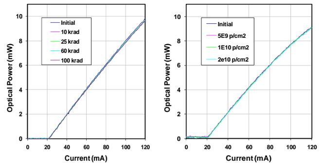
Fig. 1. Optical Power-Current characteristics of lasers exposed to gamma radiation (a) and proton radiation (b) during the different test steps
