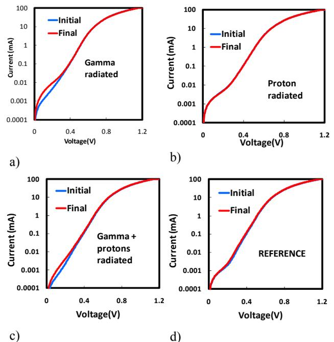
Fig. 4. Subthreshold Current-Voltage characteristics of lasers exposed to gamma radiation (a), proton radiation (b), gamma and proton radiation (c), and reference sample (d)
