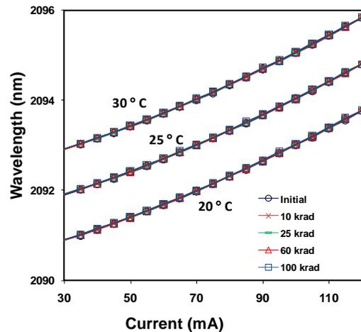
Fig. 2. Emission wavelength as a function of current at three different temperatures for a lasers exposed to gamma radiation during the different test steps.
