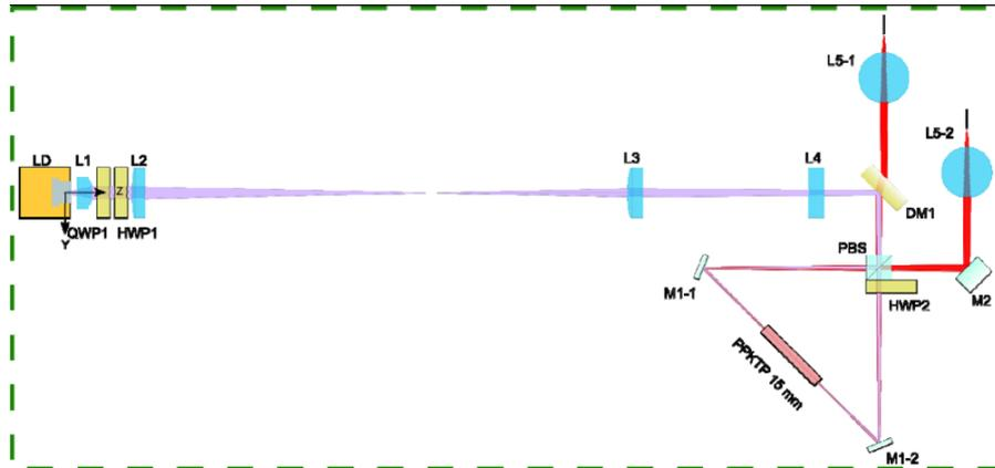
Figure 1 Scheme of the Entangled Photon Source.
