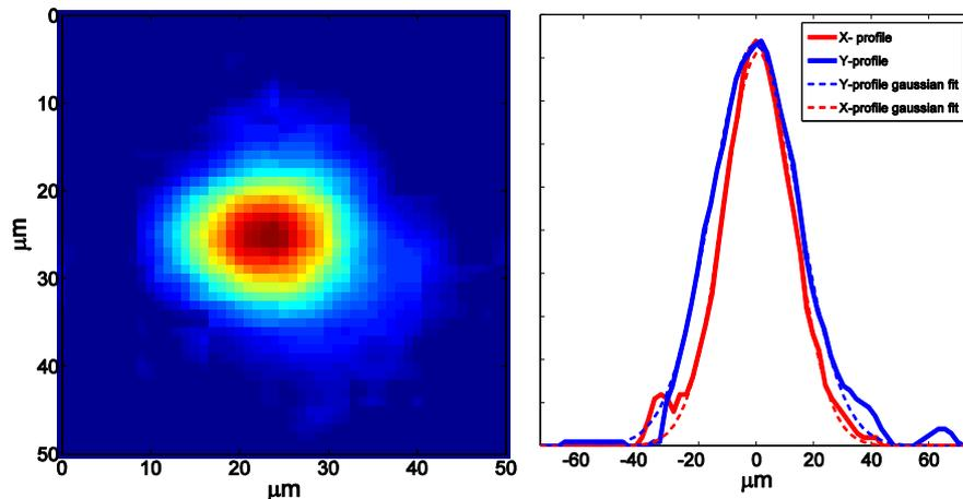
Figure 4 a) Experimental focal spot, b) profiles along x and y axes.
