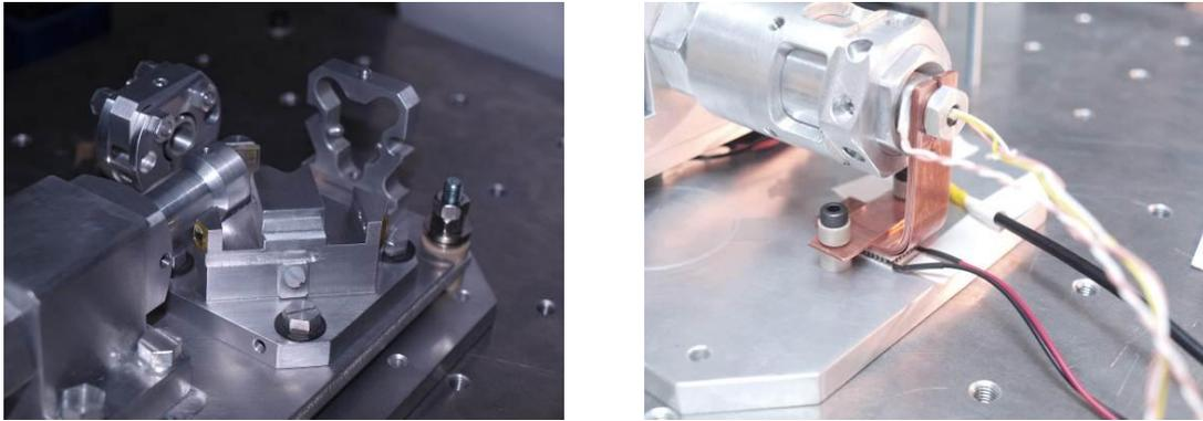
**Figure 3** a) Sagnac block and pigtailed optical fiber holder, b) Peltier module for cooling/heating the laser diode.
